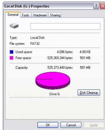
Figure 5-17 WindowsXP properties window for the new FAT32 partition
