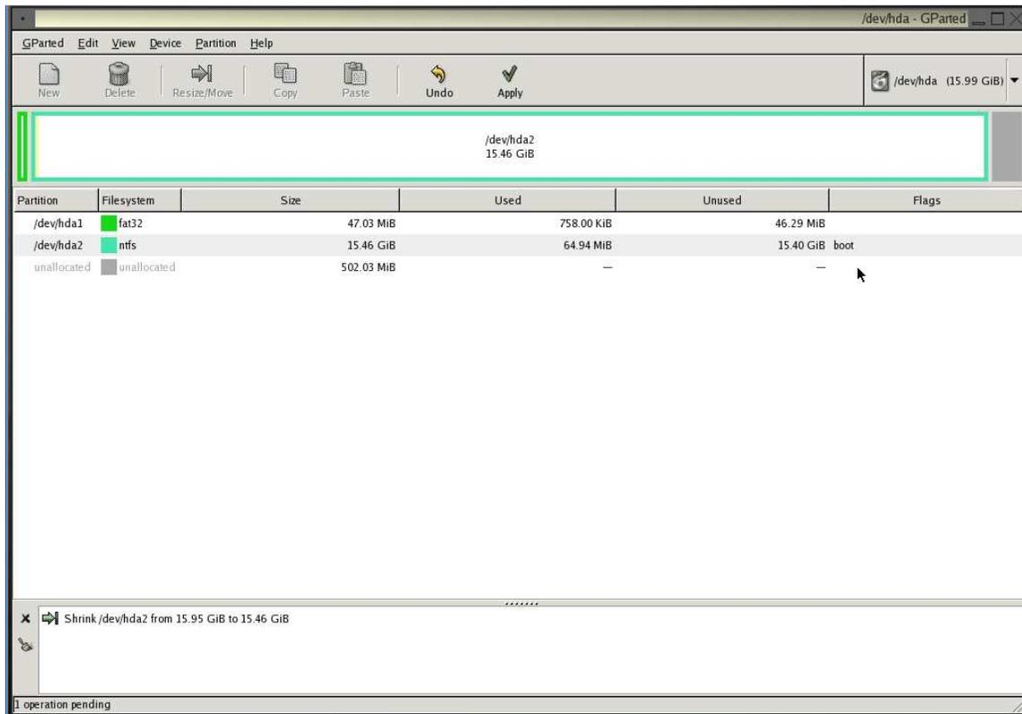
**Figure 5-5** GParted window after resizing the NTFS partition.
